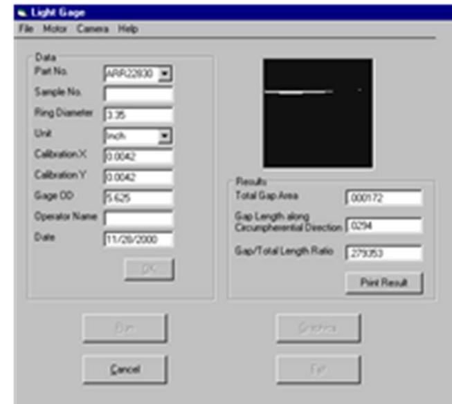
Computer screen shows numerical results for each ring data stored available to call-up, display, print, or send to data collection system
